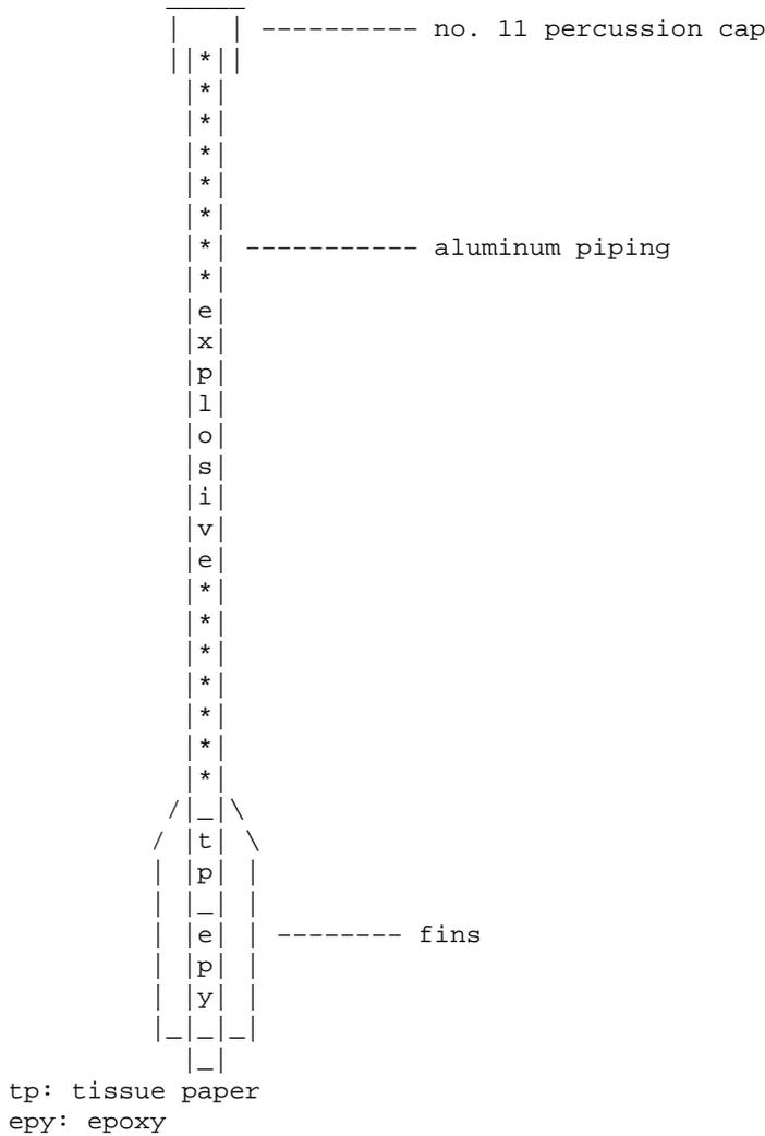
When the arrow or bolt strikes a hard surface, the percussion cap explodes, igniting or detonating the explosive.
