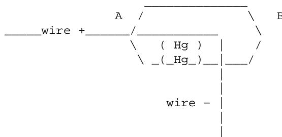
When the drop of mercury ("Hg" is mercury's atomic symbol) touches both contacts, current flows through the switch. If this particular switch was in its present position, A—B, current would be flowing, since the mercury can touch both contacts in the horizontal position.
