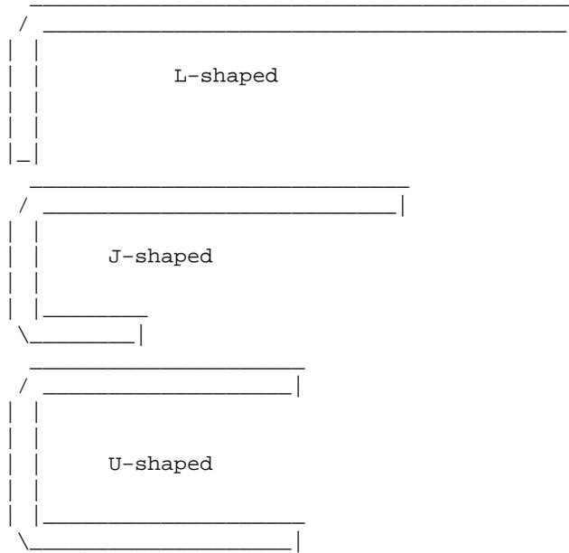
All of these devices should be used to hook the latch of a door and pull the latch out of its hole. The folds in the lockpicks will be between the door and the wall, and so the device will not unfold, if it is made properly.
