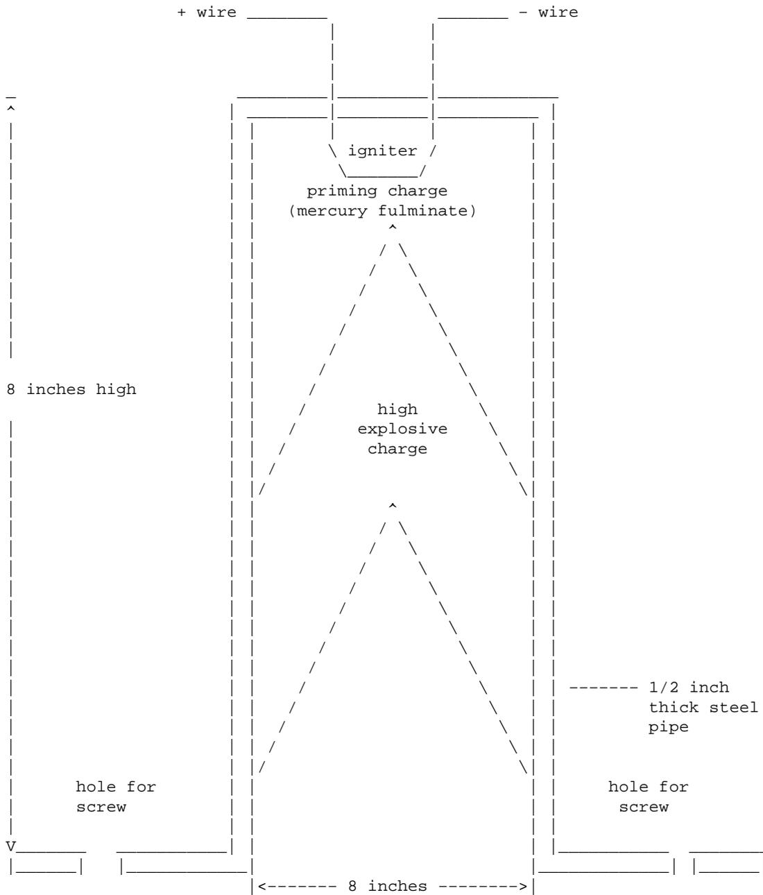
If a device such as this is screwed to a safe, for example, it would direct most of the explosive force at a point about 1 inch away from the opening of the pipe. The basis for shaped charges is a cone-shaped opening in the explosive material. This cone should have an angle of 45 degrees. A device such as this one could also be attached to a metal surface with a powerful electromagnet.
