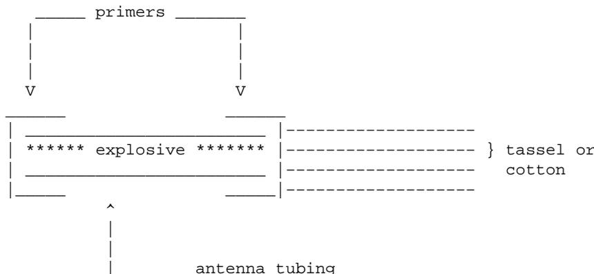
The front primer is attached to the tubing with a drop of super glue. The tubing is then filled with an explosive, and the rear primer is glued on. Finally, a tassel, or a small piece of cotton is glued to the rear primer, to insure that the projectile strikes on the front primer. The entire projectile should be about 3/4 of an inch long.
