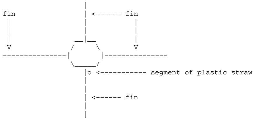
By cutting a coat hanger at the indicated arrows, and bending it, a launch rod can be made. After a fuse is inserted in the engine, the rocket is simply slid down the launch rod, which is put through the segment of plastic straw. The rocket should slide easily along a coathanger, such as the one illustrated below:
