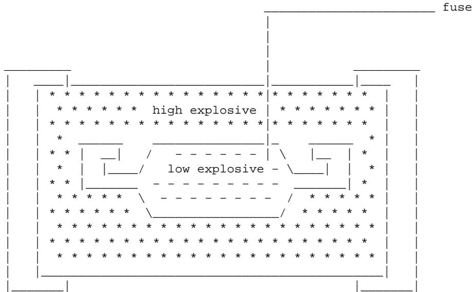
If the large high explosive container is small, such as a CO2 cartridge, then a segment of a hollow radio antenna can be made into a low-order pipe bomb, which can be fitted with a fuse, and inserted into the CO2 cartridge.
