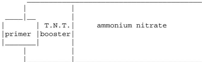
The primer explodes, detonating the T.N.T., which detonates, sending a tremendous shockwave through the ammonium nitrate, detonating it.
