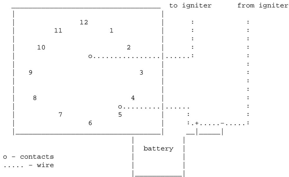
This device is set to go off in eleven hours. When the hour hand of the clock reaches the contact near the numeral 5, it will complete the circuit, allowing current to flow through the igniter or squib.
